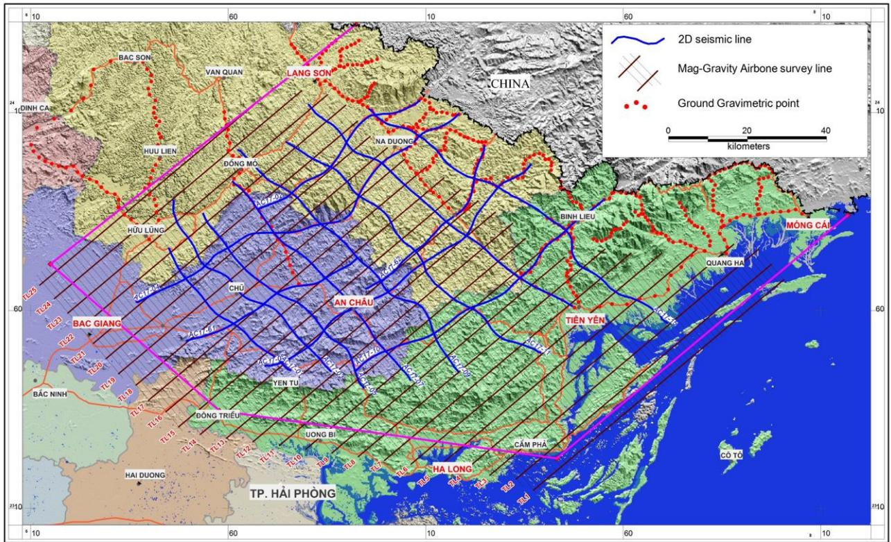
Figure 2. Seismic acquisition lines and Mag-Gravity survey lines in An Chau trough.
