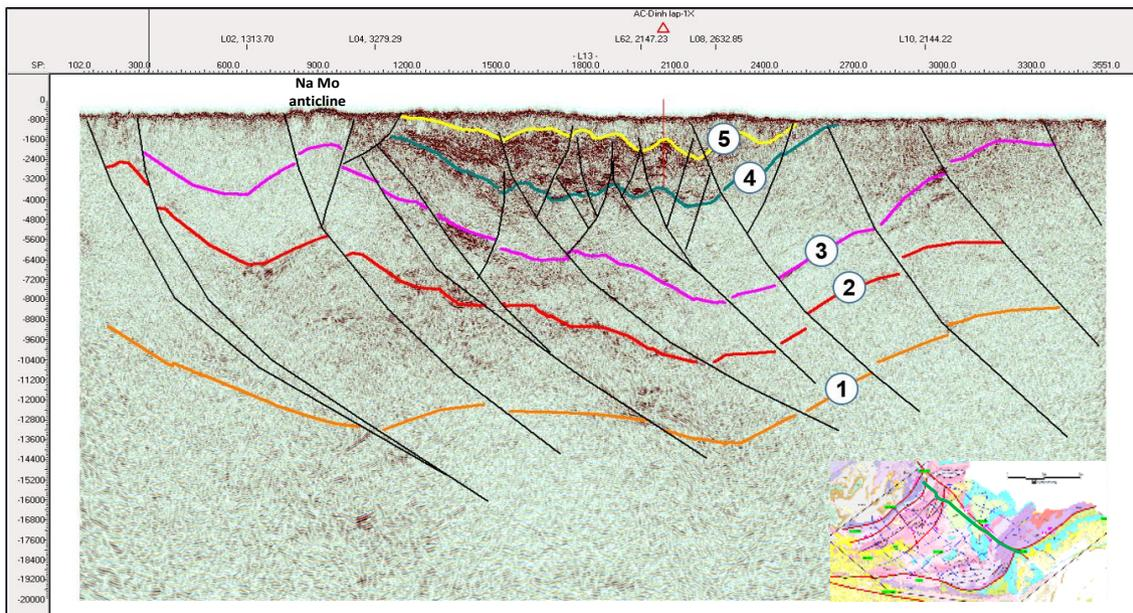
Figure 8. Fault systems, fault characters and folds defined on seismic data.
