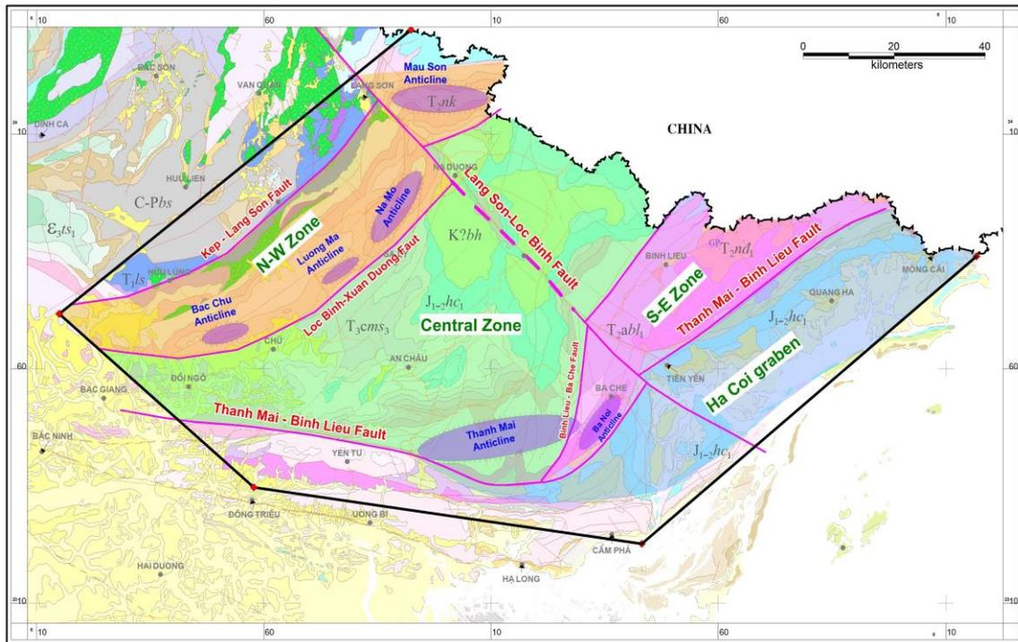
Figure 1. Geological map and structural zoning of An Chau trough.
